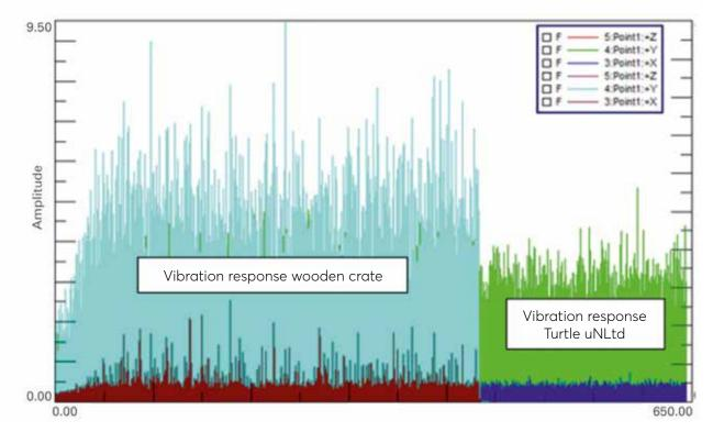
The measured results show that, where the stimulus remains equal, the middle point of the canvas of the painting vibrates, when it's packed inside the Turtle crate, with only 50% of the vibrational amplitude which occurs when it's packed inside the conventional wooden crate
